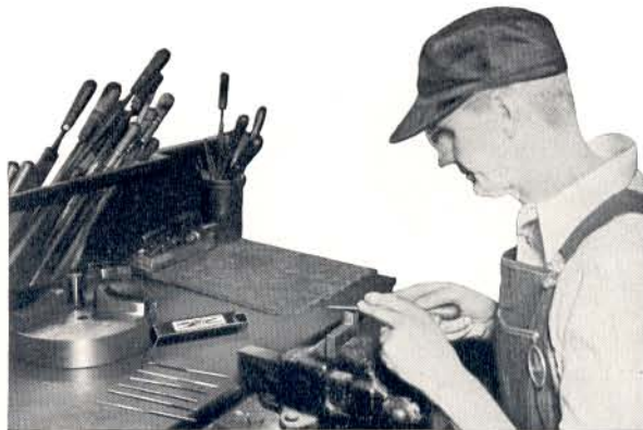
Finishing up a die with an "American Swiss" needle file.
