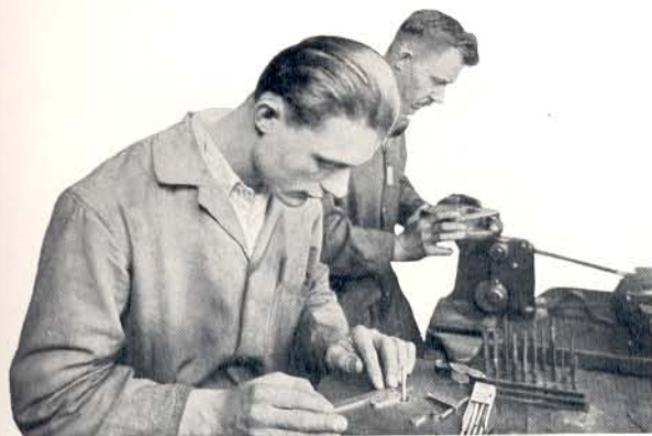
Filing small parts with "American Swiss" machine files on filing machines.
